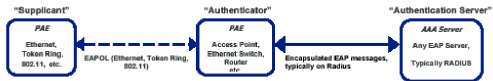
Figure 1. The IEEE 802.1x Setup
